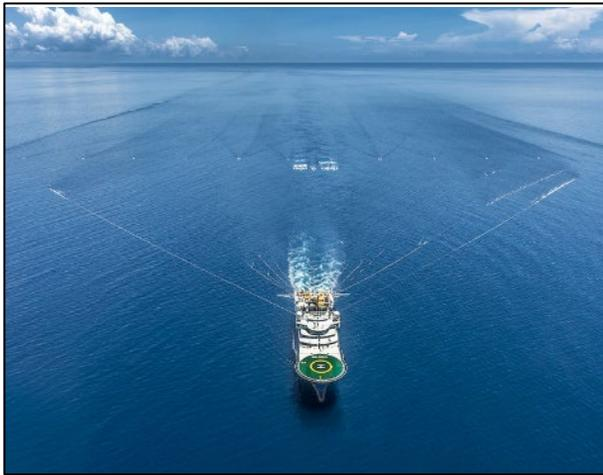
**Figure 30: 3D Seismic Survey, Offshore China (Source: Empyrean Energy, n.d., as cited in Nunami Stantec, 2018b)**
